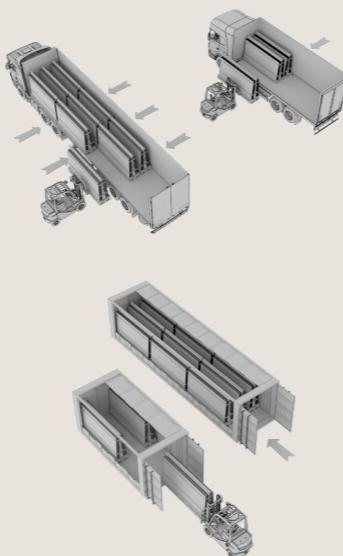
The trestle shall always be carried in a symmetrical way, and only one at a time to prevent any instability or collapse issues.
